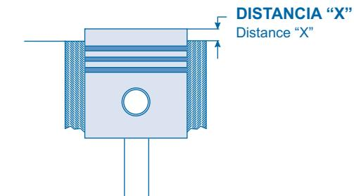
In order to keep the compression relationships steady, the gasket thickness choice is in function of piston exposure in reference to cylinder block plane indicated as distance "X" in the diagram.
